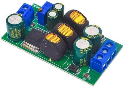
20W DC-DC Boost-Buck module with dual output Type: DD39AJPA
