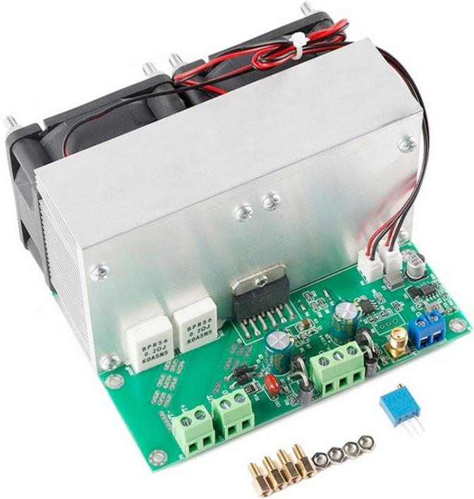
OPA549 Power-OP-Amp Module with large Heatsink (there may be two different version available, constant voltage and constant current, I'm not sure)
